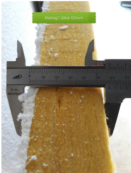
Set-up: 5 mm Power Acoustics 50 mm thick Sonaboard
