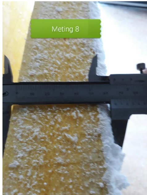
Set-up: 5 mm Power Acoustics 60 mm thick Sonaboard
